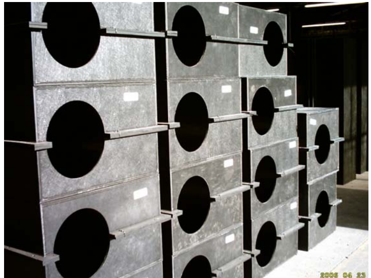
Part of the production run of 126 No. bespoke Electrical isolation box's
