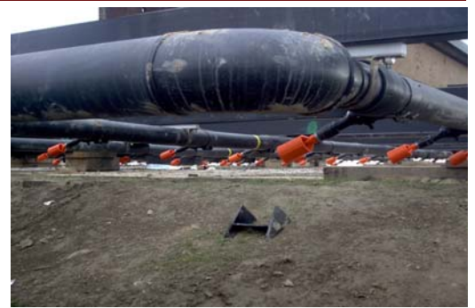
Section of the barge showing blower nozzles.
